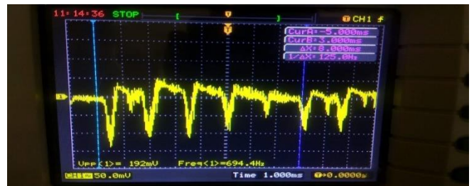
Figure 3: Noise signal at photodiode
