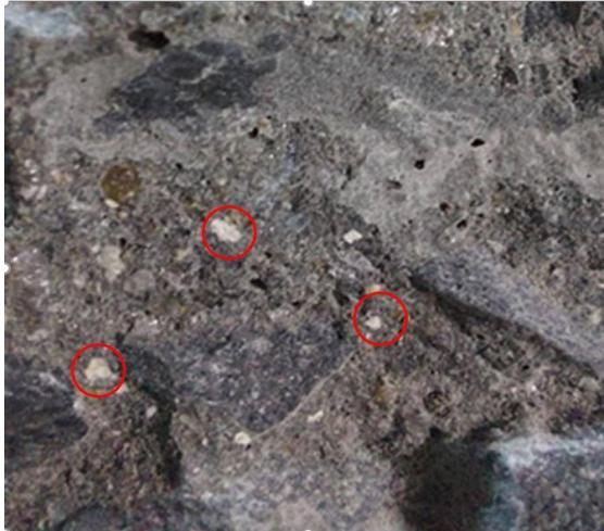
Fig. 5. The inner surface of the latex-sludge concrete.
