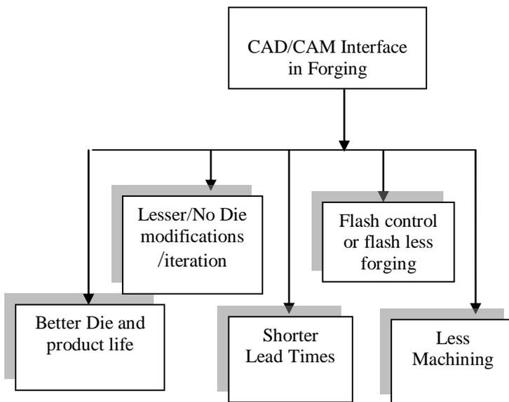
Fig1 Advantages of CAD/CAM in Forging Die-Design
