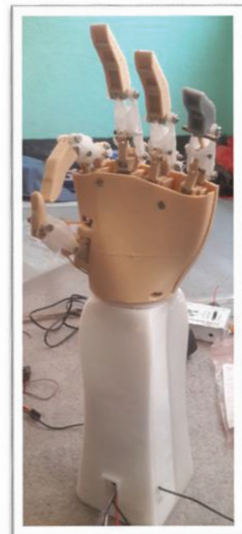
Fig 6. 3D printed prototype of prosthetic hand showing pinch operation (left) and backside view (right)
