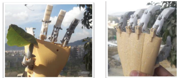
Fig 6. 3D printed prototype of prosthetic hand showing pinch operation (left) and backside view (right)
