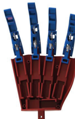
Fig 2. Rendered 3D model of the lower palm showing motor holding sockets
