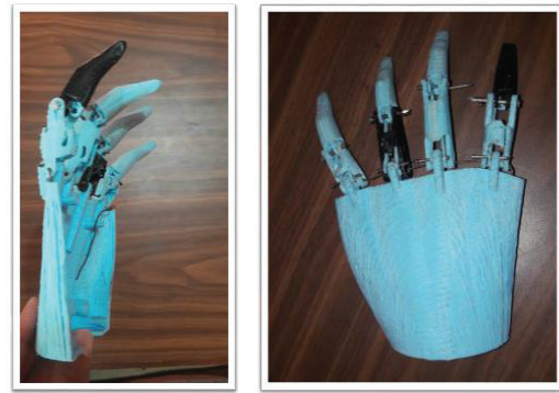
Fig 5. First 3D printed prototype of the lower palm and fingers: side view (left) and front view (right)
