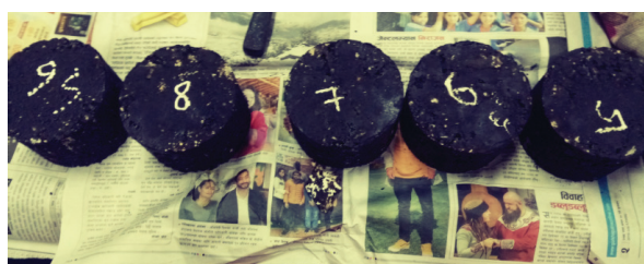
Fig. 6. Marshall sample of virgin mix
