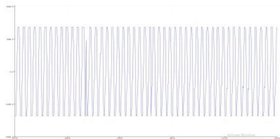
Figure 10 Random Signal when headset is not placed in head
