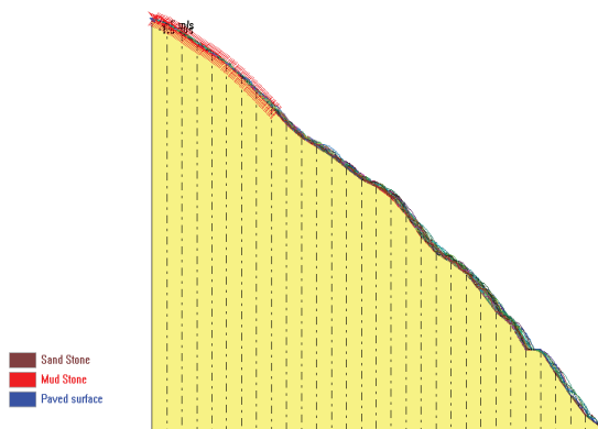
Fig. 7. Showing Rock fall simulation on first profile without barrier system
