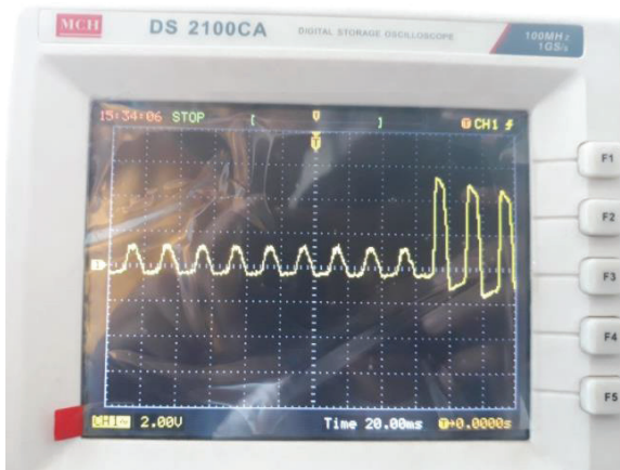
Fig.4. The transition from high to low input
