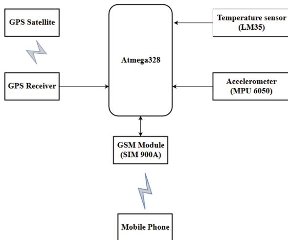
Fig. 3. Block Diagram of system
