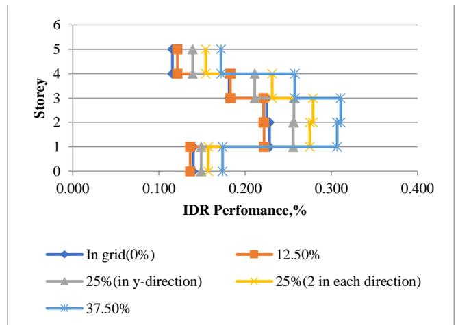
Fig. 8. Inter storey Drift EQy
