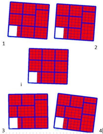
Fig. 4. Deflected shape of different models in mode 3
